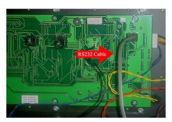
... This cable will also attach to the display board, as shown.
